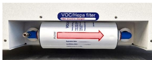
Figura 12.3 Filtru COV/HEPA corect instalat
